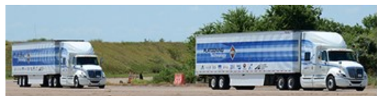
Cooperative Truck Platooning using V2V DSRC (US)
